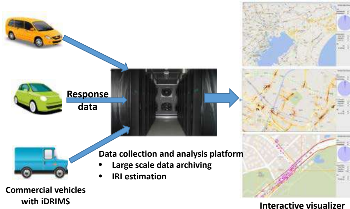
Fig. Display road condition with a heat map
